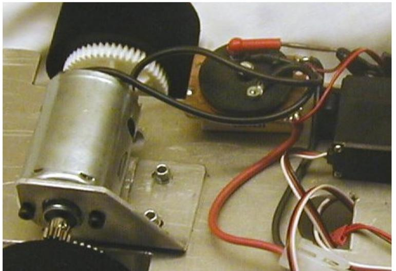
An alternative to the use of resistors, which draw current from the battery, is to develop an electronic speed controller for yourselves.
